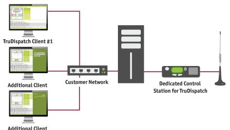
The server interfaces to the radio system using a dedicated control station while the TruDispatch Manager administers the channels, and audio stream. The TruDispatch Console software can be installed on any networked computer to communicate back with the server to place/receive calls and texts messages, and access recorded data and logs.
