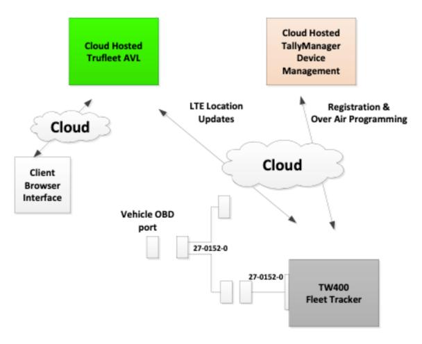
Figure 2 Simplified System Diagram – cloud hosted
